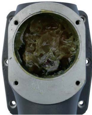
Figure 3 new grease example (before any single use)
